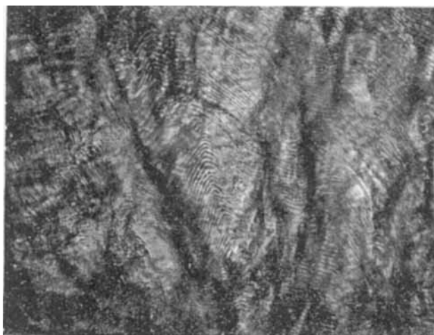
B. Twenty micron thick section of solid PBLG: 3,3'dimethylbiphenyl 7 : 3, S = 2 microns. In both photographs the microscope was used with crossed polars to improve contrast.
